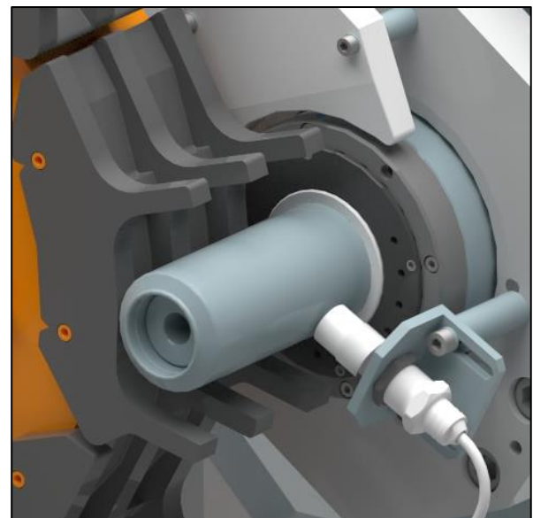
Fig. 2 – Short Can Sensor in Position with Fixture Removed
